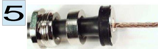
Remove the copper foil and the dielectric with a knife.
