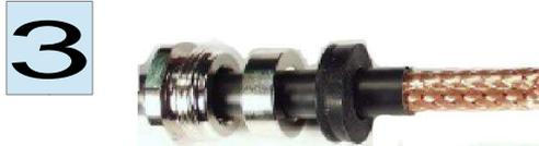
Remove 20 mm of the outer sheath with a knife.
