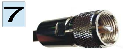
Carefully solder the inner conductor at the tip.
