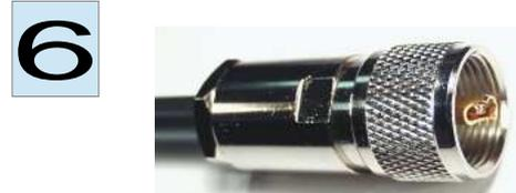
The prepared cable tail has to be carefully inserted into the housing until stop. Tighten the clamping nut finger tight with two open-ended spanners 16 mm.
